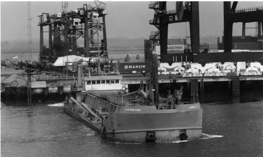
Figure 2.23 A trailing suction hopper dredger dredging a berth
